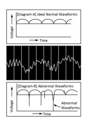
This product uses Samarium-based rare earth magnet for field magnetic flux source and it keeps to generate high magnetic flux constantly and stably. The coil generates alternating current (AC) by driving MovingCoil-Type Roter but since the commutator rectifies the voltage and outputs it by converting to direct current (DC) through a brush, output waveforms would be as shown in [Drawing-A] ideally.
