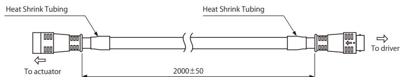
※ The length that can be guaranteed with the open collector type is up to 2.5 m. When ordering an open collector type actuator and selecting this MA-175-020, please specify the 200 mm long cable by adding 03 to the last digit of the model number.
