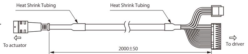
※ The length that can be guaranteed with the open collector type is up to 2.5 m. When ordering an open collector type actuator and selecting this MA-171-020, please specify the 200 mm long cable by adding 03 to the last digit of the model number.
